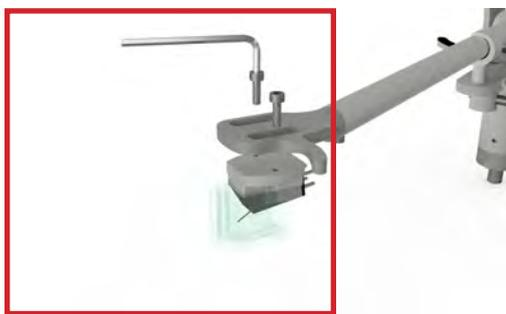
Pic. 8: Mounting the cartridge
