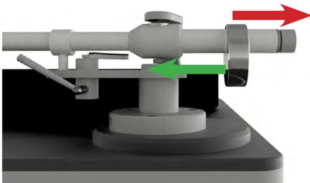
Caution: Please hold the tonearm tube while rotating the counterweight to avoid any damages.
