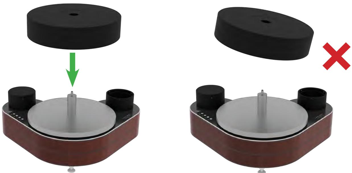
**Pic. 12:** Mounting the POM platter
